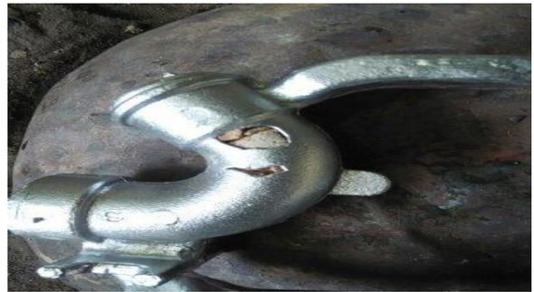
Figure 7: Defective casting part
