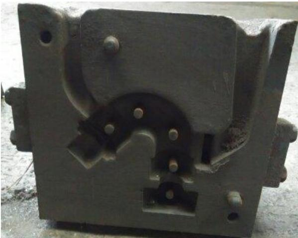
Figure 5: Second part of the mould
