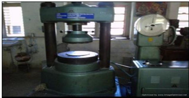
Figure: Compression strength test for Brick
