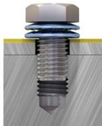
Figure 2: Tapped hole showing thread engagement
