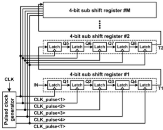
Figure 2: Conventional method 2 shift register using SSASPL
