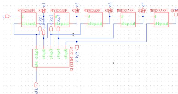
Figure 15: Schematic of proposed 4bit shift register.
