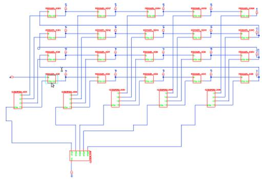
Figure 17: Schematic of proposed 16 bit shift register.
