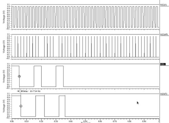
Figure 10: Simulation results of TSPC pulsed latch
