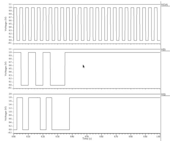
Figure 6: Simulation results of conventional PPCFF Master-slave flip-flop
