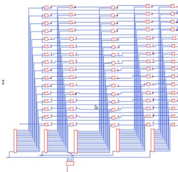
Figure 19: Schematic of proposed 64 bit shift register.
