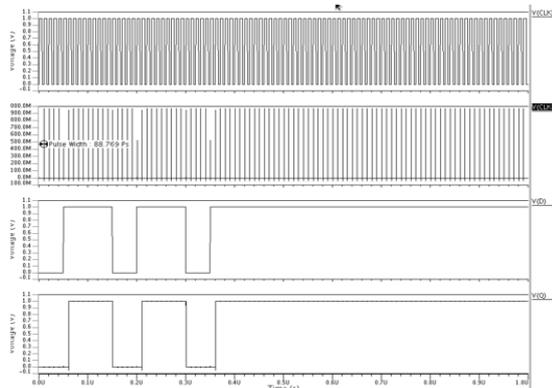
Figure 8: Simulation waveforms of SSASPL pulsed latch
