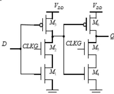
Figure 4: True Single Phase clocked pulsed latch
