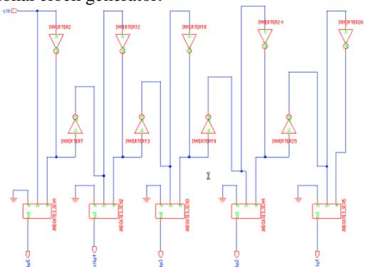
Figure 13: Schematic of proposed clock generator
