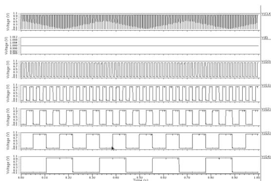
**Figure 26:** Simulation results of Synchronous up counter
