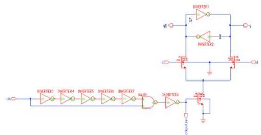
Figure 7: Schematic of conventional method 2 SSASPL Pulsed latch
