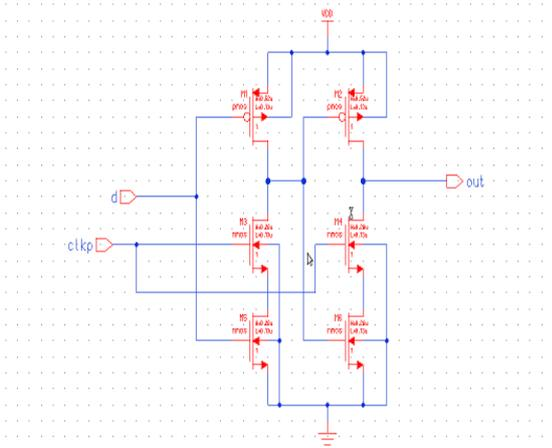
Figure 9: Schematic of proposed TSPC pulsed latch
