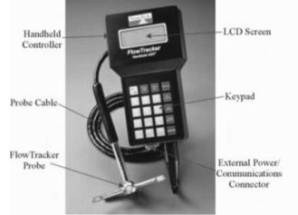
Figure 1: Flow Tracker with 2D Probe
