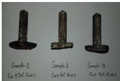
Figure 2: Pictorial view casting of samples
