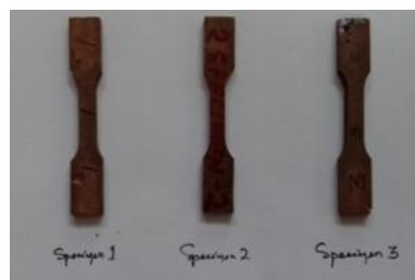
Figure 5: Standard samples for tensile test
