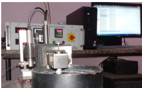
Figure 3: Pin on disc apparatus set up
