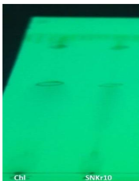
Figure 8 (b): TLC analysis of SNKr10 extracted secondary metabolic compounds visualization by keeping TLC plates under UV light
