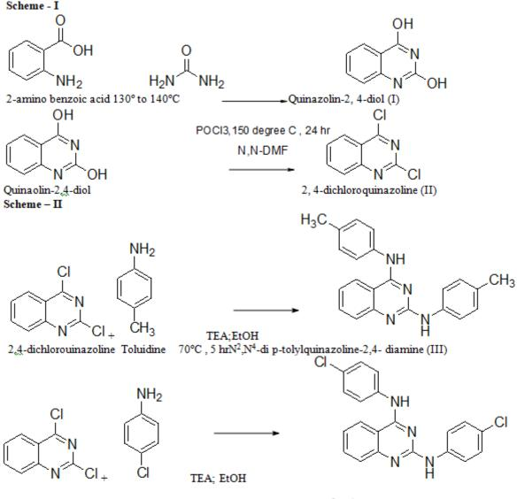
2, 4-dichlorouinazoline P-chloroaniline 70°C , 5 hrN<sup>2</sup>, N<sup>4</sup>-bis(4-chlorophenyl) quinazoline-2,4-diamine(IV)
