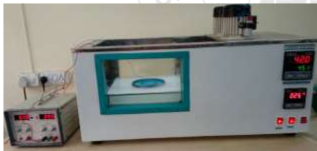
Figure 1: Photograph of setup of constant temperature bath
