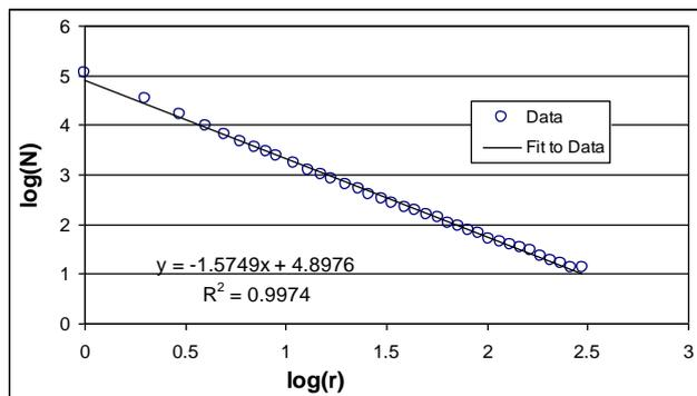
**Figure 5:** log(N) versus log (r) plot for Electrodeposit of copper from 1 M CuSO4 solution at a cell operating voltage of 6V at 50°C
