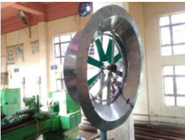
Figure 6: Experimental setup of Wind lens and Bicycle wheel wind turbine
