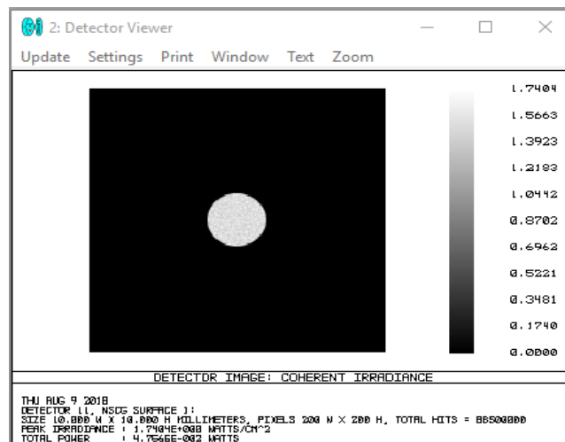
Figure 17: Detector image of the scaled interferometer
