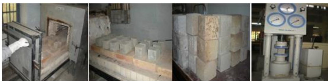
Figure 1: Temperature exposure in built furnace and testing of cubes
