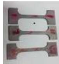
Figure 3.2: Specimen before tensile test
