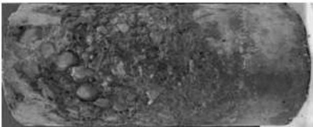
Figure 13: OPC - FA specimens after 28 days of dipping in 3.5% concentrated sodium Sulphate solution.
