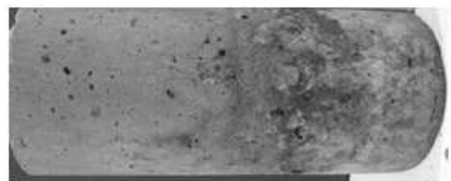
Figure 10: Specimens after 14 days of immersion in 3.5% concentrated sodium Sulphate solution.
