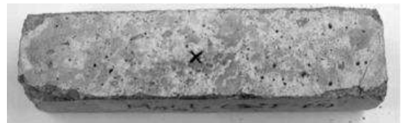
Figure 14: Specimens after 28 th day immersion in 4% concentrated Chloride solution under exposure to wet and dry condition
