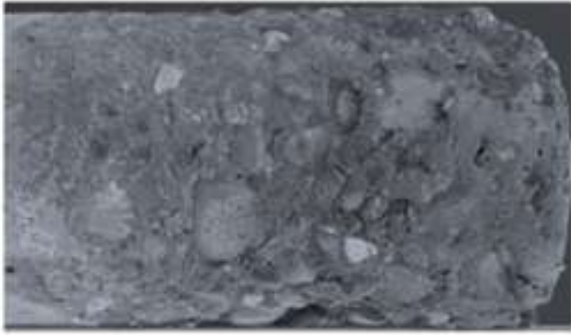
Figure 11: Concrete cylinder after 28 days immersion in salt water under wet – dry cycles
