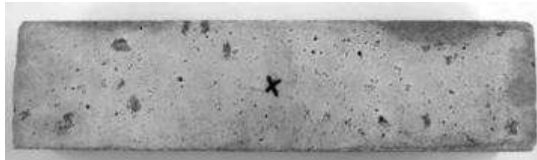
Figure 16: Specimens after 28 th day of immersion in 2% concentrated Chloride Solution
