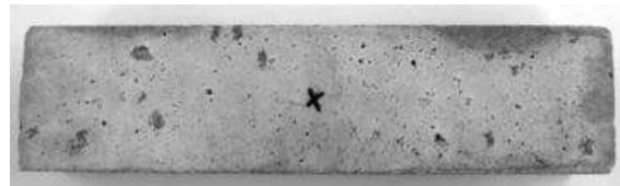
Figure 13: Concrete beam after 28 th day dipping in a 2% concentrated Chloride solution with no exposure to freeze and thaw or wet and dry cycles
