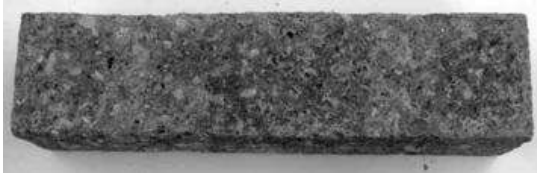
Figure 17: Specimens after 28 th day of immersion in 6% concentrated Chloride solution
