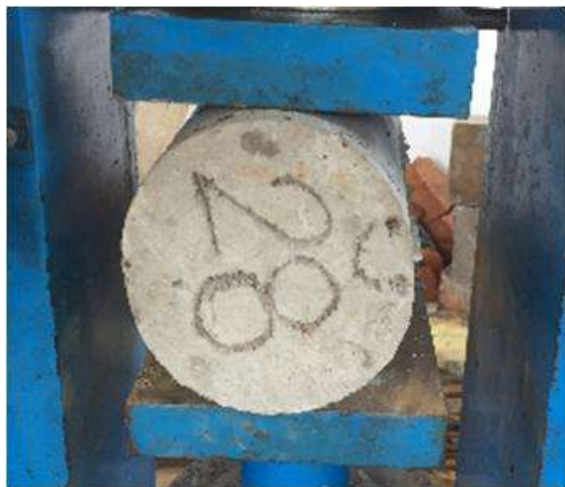
Figure 4: Cylinder placed in CTM
