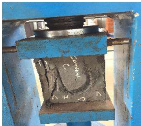
Figure 2: Cube placed in CTM
