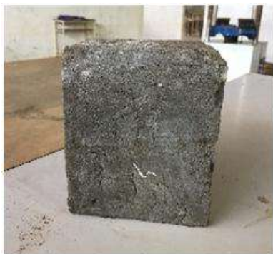
Figure 11: Specimen after acid test
