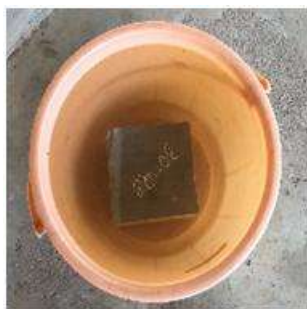
Figure 10: Specimen immersed in H 2 SO 4 solutions
