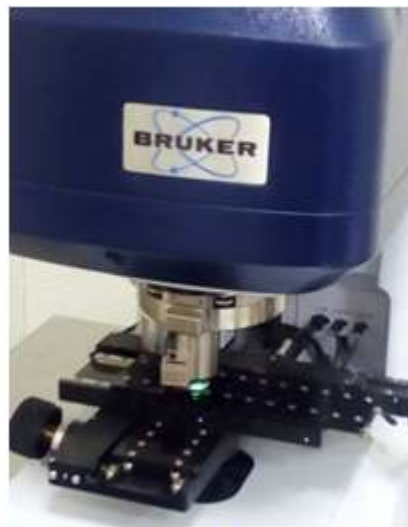
Figure 3: Profiler used for roughness work
