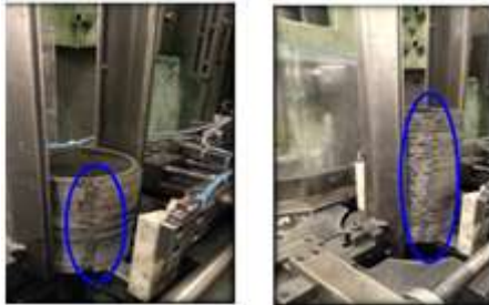
Figure 13: I-Section Rings Loading Method in Lapping Process before and After the Design Improvement
