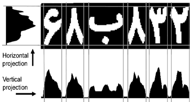
Figure 3: Character extraction using the horizontal and vertical projection method
