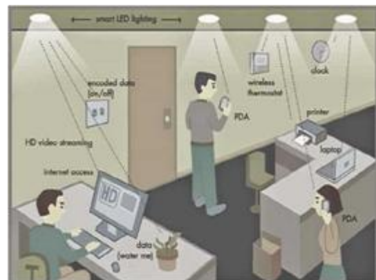
Figure 6: Li-Fi system connecting devices in a room
