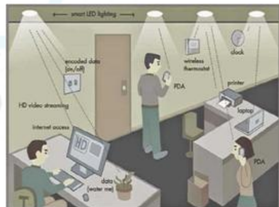
Figure 6: Li-Fi system connecting devices in a room
