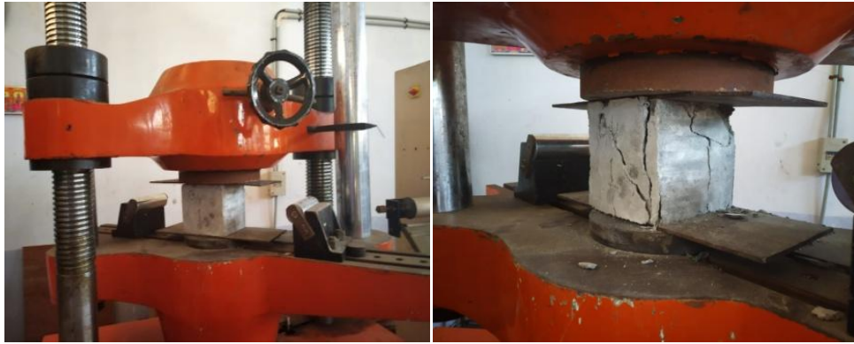
Figure 8: Compressive Strength of Cubes and Crack Pattern
