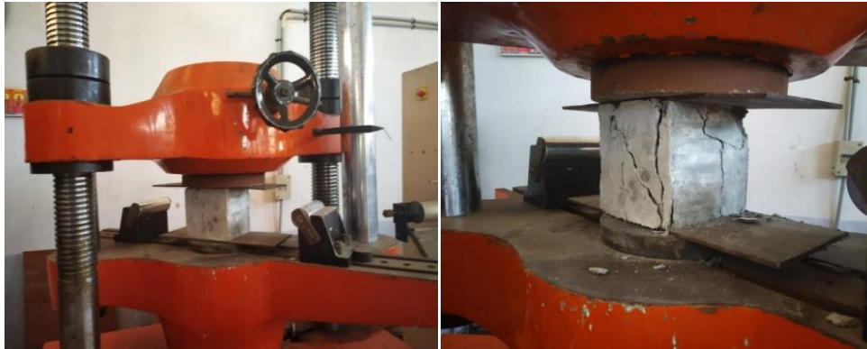
Figure 8: Compressive Strength of Cubes and Crack Pattern
