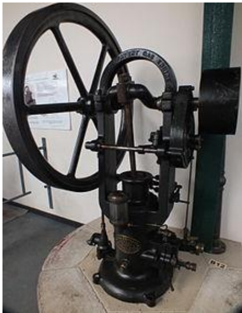
Figure 1: Griffin six stroke engine
