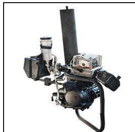
Figure 4: Niykado six stroke engine
