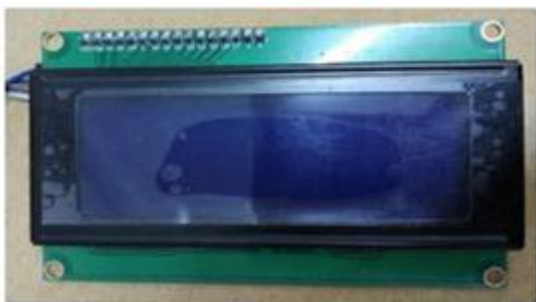
Figure 4: I2C LCD2004 Display
