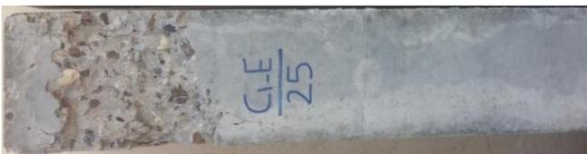
**Figure 15:** failure mode of (Specimen C1-E-25) spalling out of concrete cover
