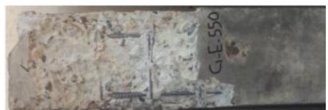
**Figure 22:** failure mode of (Specimen C1-E-550) spalling out of concrete cover
