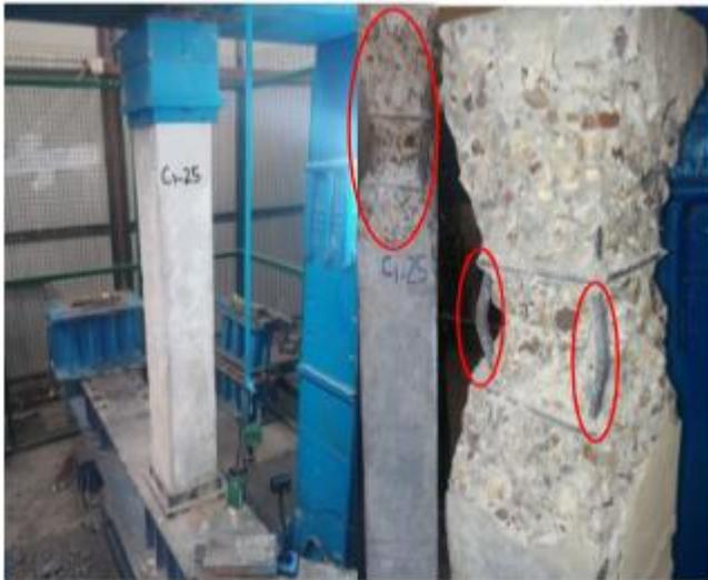
**Figure 13:** failure mode of (Specimen C1-25) crushing of concrete and local buckling of steel
