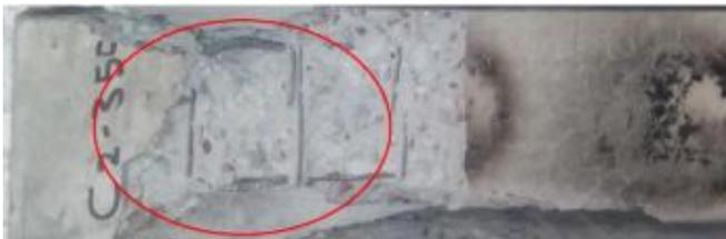
**Figure 19:** failure mode of (Specimen C2-350) crushing of concrete and local buckling for steel
