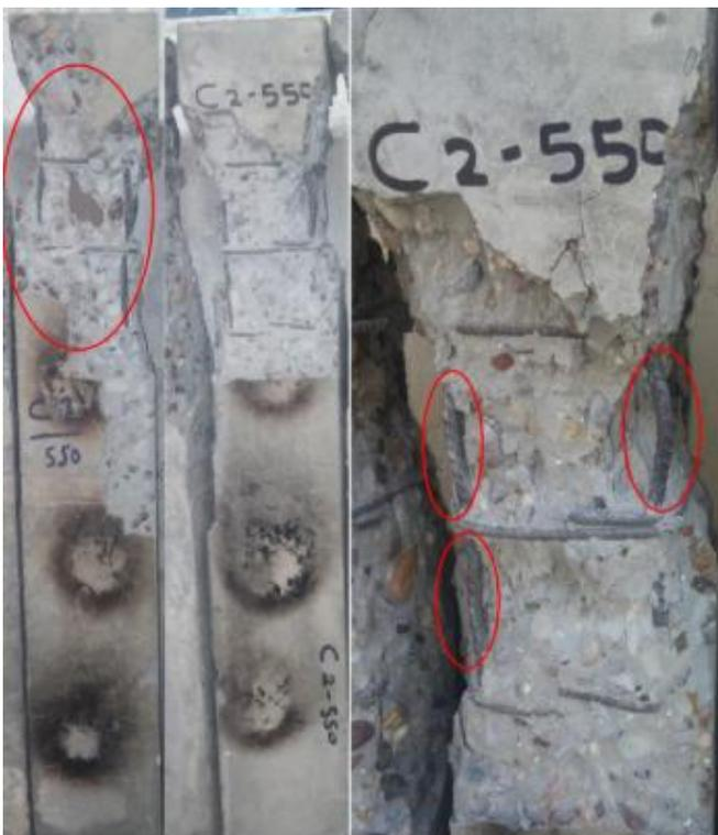
**Figure 20:** failure mode of (Specimen C2-550) crushing of concrete and local buckling for steel
