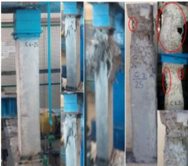
**Figure 14:** failure mode of (Specimen C2-25) ) crushing of concrete and local buckling of steel
