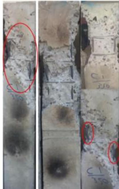
**Figure 16:** failure mode of (Specimen C1-350) crushing of concrete and local buckling for steel
