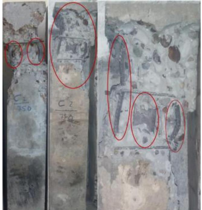
**Figure 21:** Failure mode of (Specimen C2-750) crushing of concrete and local buckling for steel
