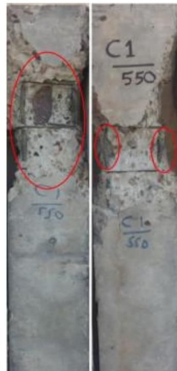
**Figure 17:** failure mode of (Specimen C1-550) crushing of concrete and local buckling for steel
