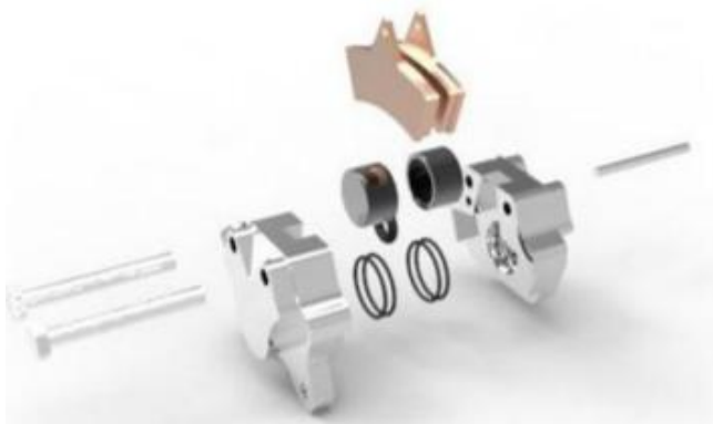
Figure 1:- Exploded View of Brake Caliper
