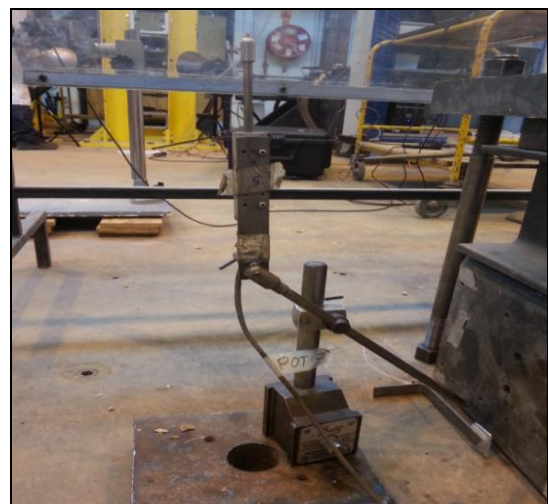
Figure 3: LVDT Device Located on the Base.
