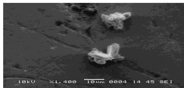
Figure 3.1.10: SEM picture of calcium oxalate monohydrate hexagonal at Ca/OA molar ratio 2.0
